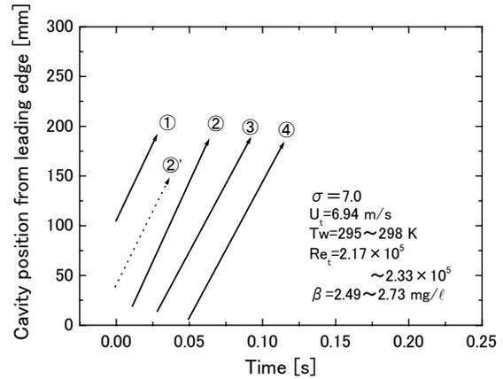
**Fig.9 Loci of shedding cavities and sub-cavities based on Fig.8**
