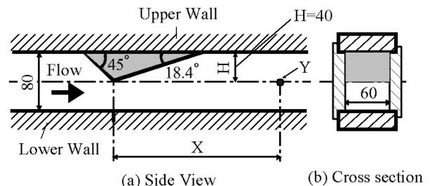
Fig.1 Convergent-divergent channel
