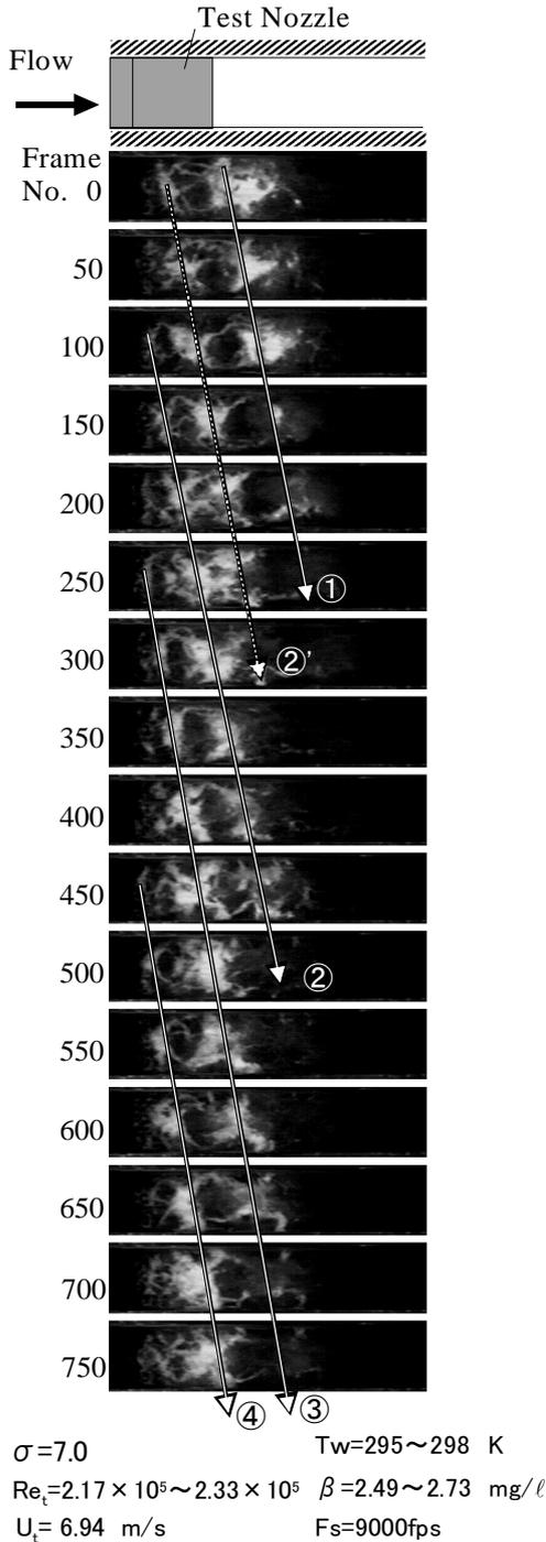
**Fig.8 Behavior of vortex cavities at higher cavitation number: span-view observation**
