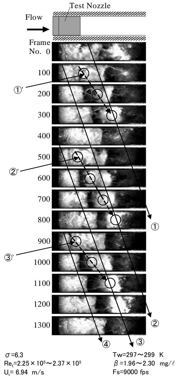
**Fig.5 Shedding behavior of cavitation cloud : span-view observation**
