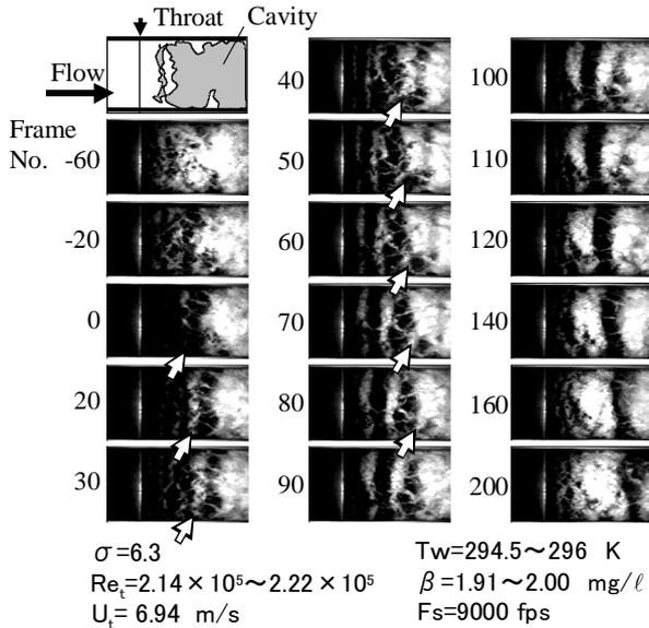
**Fig.6 Details of vortex-cavity motion just behind nozzle throat: span-view observation**
