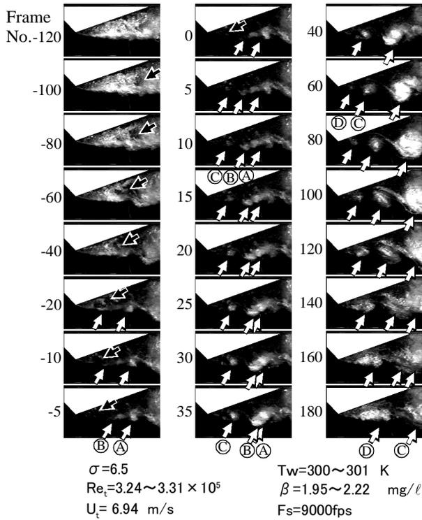
**Fig.4 Details of vortex-cavity motion just behind nozzle throat: side-view observation**
