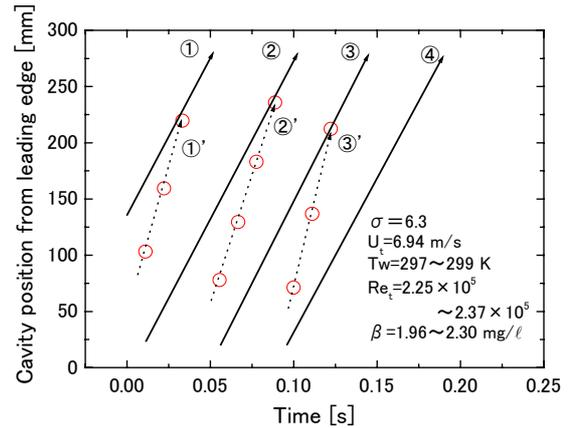
**Fig.7 Loci of shedding cavities and sub-cavities based on Fig.5**
