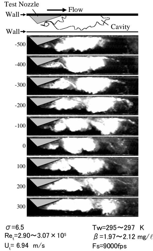
**Fig.3 Shedding behavior of cavitation cloud : side-view observation**
