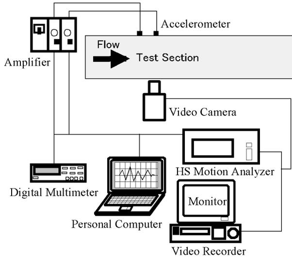
**Fig.2 Measurement and observation system**
